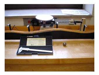
**Example 2**: A steelball with mass  $m=0.44\,\mathrm{kg}$  and radius  $r=1.0\,\mathrm{cm}$  moves along a rollercoaster. Seven photogates are placed along the track at different heights  $h_i$  from the base of the track; we measure the time intervals  $\Delta t_i$  for the steel ball to pass through each photogate,
